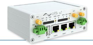
3G UMTS/HSPA routers, UR5i v2 series, are used to wirelessly connect various equipment and devices via Ethernet 10/100 to the Internet or intranet. High data transfer speed of up to 14.4 Mbit/s (download) and upload speed up to 5.76 Mbit/s, make it an ideal wireless solution for traffic and security camera systems, individual computers, LAN networks, automatic teller machines (ATM) and other self-service terminals, etc.
