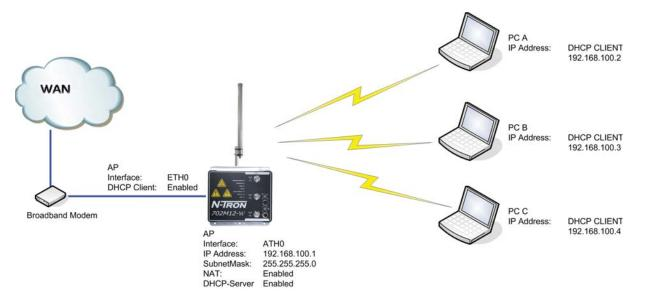
The N-TRON 702M12-W configured as a router can act as a DHCP server and supports the Network Address Translation (Masquerading) feature which is widely used by Access Points. This automates the assigning of IP addresses to devices as they connect. NAT will act as a firewall between LAN and WLAN networks. Additional firewall settings can be configured for layer 3 packet filtering and access control in Router mode.
