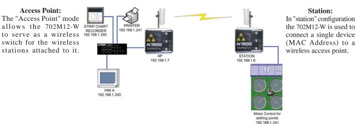
For added security, the 702M12-W supports WEP, WPA<sup>TM</sup>, and WPA2<sup>TM</sup>. WPA and WPA2, TKIP (Temporal Key Integrity Protocol) and CCMP (Counter Mode with Cipher Block Chaining Message Authentication Code Protocol) are available.
