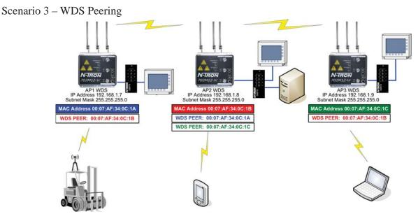
In this scenairio, each 702M12-W has been configured as a peer of selected other 702M12-W(s) by using the MAC Addresses of the select unit(s). This allows forklifts or other mobile wireless devices to maintain communication seamlessly as they move from the area covered by one 702M12-W into the area covered by the next 702M12-W.
