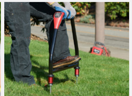
Pinpoint fault location by using the AF-600-EUR with the UAT-600-TE Transmitter
