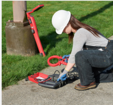
The Transmitter will automatically change modes based on which accessory is plugged in
