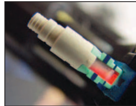
A light can be seen through the clear window on the connector body until a fiber has been properly terminated.
