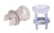
The slotted screw with knurled nut provides effective shield bonding of large aircore and filled service wires up to ½" shield O.D. (11, 16 and 25 pairs) to a ground wire or ground stud. Can also be used to bond the two pieces of butt spliced service drop within a buried service drop closure.
