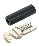
The one-piece clip, bonds or grounds the shield of a service wire or small cable up to ¼" O.D. or 3/8" O.D. at station protectors, pedestals and similar terminations. Low resistance path to ground prevents stray electromagnetic interference from inducing noise or cross talk on cable pairs and provides a ground circuit path from the shield to the ground protector.
