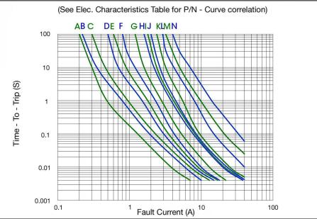
The Average Time Current Characteristic Curve and Temperature Rerating Curve are affected by a number of variables and these curves are provided for guidance only.
