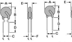
Fig.1 Lead Size : 24AWG Φ 0.51 mm Diameter
