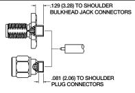
Clean all debris from the prepared cable and insert the cable into the connect making sure that the cable jacket bottoms out against the internal shoulder of connector body.
