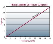
Phase stability is defined as the change in phase when the cable is bent 360 degrees around its minimum bend radius.
