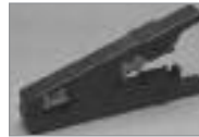
4" Universal UTP Stripping Tool for Round or Flat Wire and UTP Cable from 3.5 mm-9 mm max. Even irregular outshape of insulation can be put into the V and U slots. Strips 2, 4, 6 & 8 Conductor. Flat or Round, Solid or Stranded Cable.
