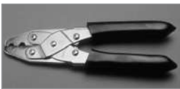
Economy Hex Crimping Tool for RG-6 & RG-59. Economy packaged in non-retail box.
