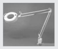
This lamp has a a strong extendable 45" white enameled steel arm for precise positioning and a heavy-duty clamp for desk edge, table or fixed horizontal surface mounting. It is designed with a 5" diameter lens for extra magnification for reading, hobbies or close work to prevent eye strain, a 22W fluorescent circular tube for work area illumination, and a 3 conductor cord set with outlet. Lamp is individually packaged in an attractive Retail Box and is sold in cases of four.
