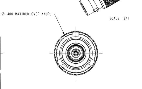
2. SUBMINIATURE CONCENTRIC TWINAX/TRIAX FEED THRU ADAPTER (TRS RECEPTACLE TYPE)
