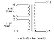
Primaries are designed to be used simultaneously. That is, they must be used either series or parallel connected (as one winding).
