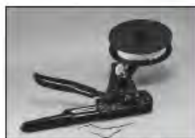
Contact Crimp Hand Tool (300 Contact Reel)
