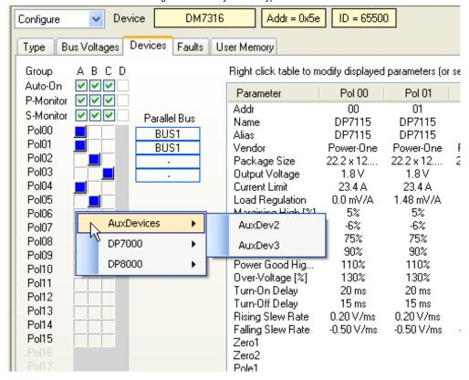
Turn-on and turn-off delays can be programmed for each Auxiliary Device as shown in Figure 7. Timing of turn-on and turn-off events can be synchronized between Auxiliary Devices and POL converters by programming appropriate delays for specific types of devices.
