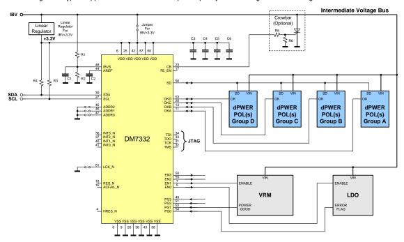
The schematic of a typical application of a DM73XX digital power manager (DPM) is shown in Figure 3. The system includes four groups of d-pwer Point Of Load converters (POLs). A group is defined as one or more POL converters interconnected via OK pins. Grouping of the POLs enables users to program advanced fault management schemes and define margining functions, monitoring, start-up behavior, and reporting conventions.
