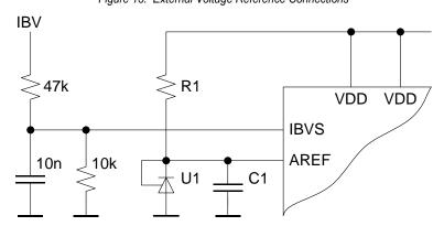
Figure 13. External Voltage Reference Connections
