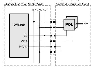
Figure 17: INTO Configured as Group A Reprogramming Trigger
