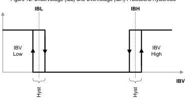
Figure 12: Undervoltage (IBL) and Overvoltage (IBH) Protections Hysteresis
