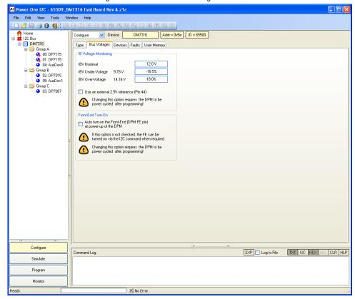
Figure 11. Intermediate Bus Configuration Window
