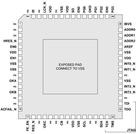
Figure 21. DM73XX Mechanical Drawing – Top View
