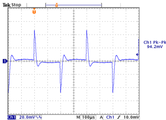
Figure 9 Transient Response with Regulation set to 0 mV/A
