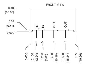
Figure 3. Mechanical Dimensions
