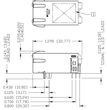
ORIGINATED BY TITLE PART NO. / DRAWING NO. STANDARD DIM [ ] METRIC DIM. JESSE LI gigabit MagJack® TOL. IN INCH AS REF. 08261X1T23-F **DATE** 2016-08-11 (12 cores, Tab Up) UNIT : INCH [mm] DRAWN BY FILE NAME 0826-1X1T-23-F SCALE: N/A JOLLY LUO .XX 08261X1T23-F\_G,DWG **DATE** 2016-08-11 ±0,010
