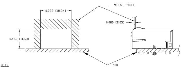
THE DISTANCE OF PANEL INSIDE SURFACE RELATIVE TO FRONT SURFACE OF PART IS ONLY A SUGGESTION. IN CASE THIS DISTANCE IS DIFFERENT, THE REQUIRED PANEL OPENING DIMENSIONS CHANGE ACCORDINGLY.
