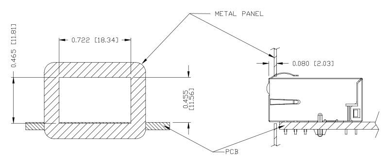
THE DISTANCE OF PANEL INSIDE SURFACE RELATIVE TO FRONT SURFACE OF PART IS ONLY A SUGGESTION. IN CASE THIS DISTANCE IS DIFFERENT, THE REQUIRED PANEL OPENING DIMENSIONS CHANGE ACCORDINGLY.
