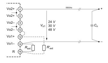
Fig. 22 Double-output models: Wiring of the R-input for output voltages 24 V, 30 V, or 48 V with both outputs in series. A ceramic capacitor (C<sub>o</sub>) across the load reduces ripple and spikes.
