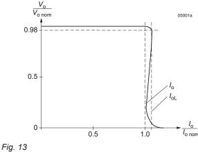
Typical output characteristic V<sub>o</sub> versus I<sub>o</sub>.
