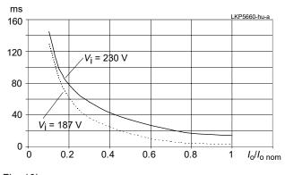
Fig. 10b Hold-up time versus output power (LKP5660-7R)
