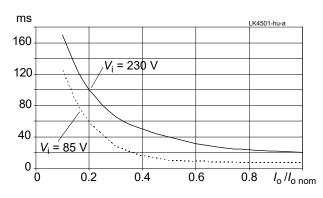
Fig. 10a Hold-up time versus output power (LK4501-7R), valid for converters with version V102 or higher.
