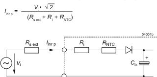
Fig. 3 Equivalent circuit diagram for input impedance.
