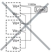
Fig.35 Example of poor wiring for parallel connection (unequal length of load lines)
