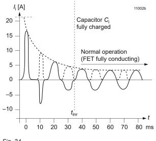
Fig. 34 Typ. inrush current with option E  $V_i = 230$  VAC,  $f_i = 50$  Hz,  $P_o = P_{o nom}$
