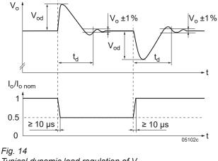
Typical dynamic load regulation of  $V_{o}$ .
