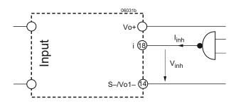
Fig. 18 Definition of V<sub>inh</sub> and I<sub>inh</sub>.
