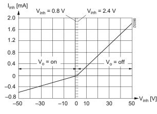
Fig. 19 Typical inhibit current I<sub>inh</sub> versus inhibit voltage V<sub>inh</sub>
