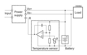
Fig. 24 Connection of a temperature sensor
