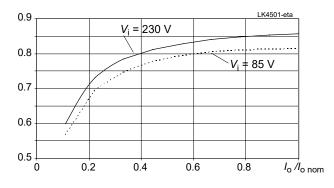
Fig. 11a Efficiency versus output current (LK4501-7R)
