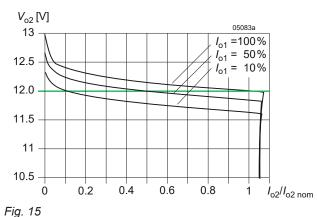
Models with 2 outputs 12 V:  $\Delta V_{o2}$  versus  $I_{o2}$  with various  $I_{o1}$  (typ).
