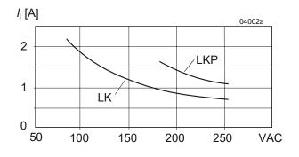
Fig. 5 Input current versus input voltage at I<sub>o nom</sub>
