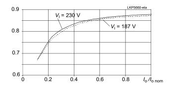
Fig. 11b Efficiency versus output current (LKP5660-7R)
