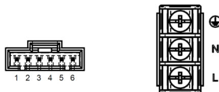
Figure 3 - LPM616 Front Panel Connectors Pinout View
