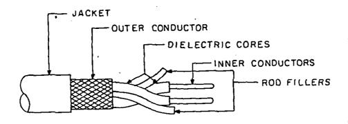
FIGURE 1. Configuration M17/176-00002 and M17/176-00003.
