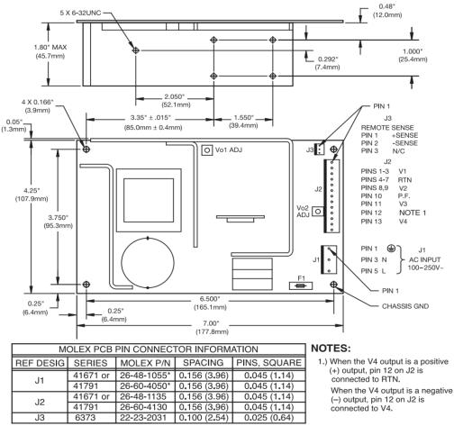
\*With pins 2 & 4 removed for double spacing.
