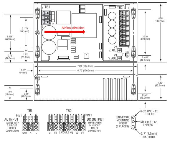
Figure 1. Mechanical Drawing
