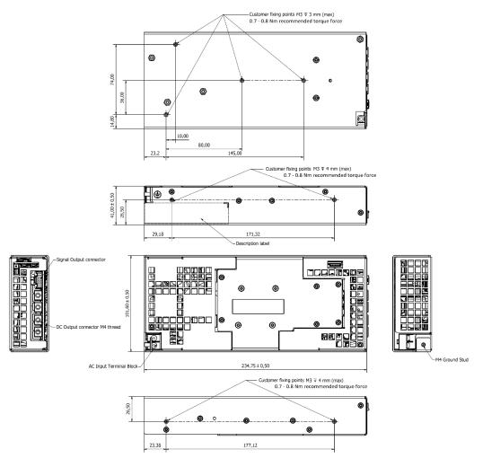
Figure 5. Mechanical Drawing - MCC750-1T24-PC / MCC750-1T48-PC Models
