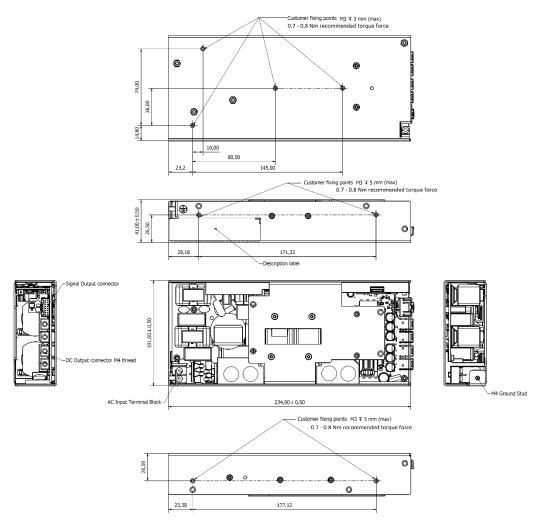
Figure 2. Mechanical Drawing - MCC750-1T24 / MCC750-1T48 Models
