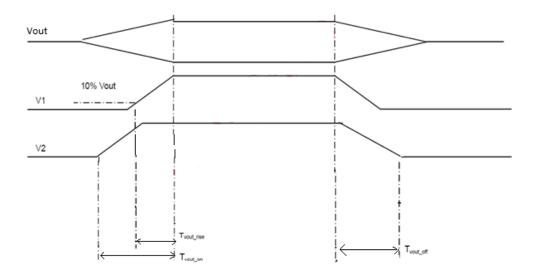
Figure 6. Output Voltage timing
