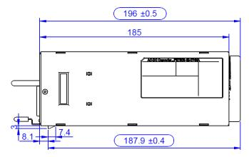
Figure 14. Mechanical Drawing-Side/Top View
