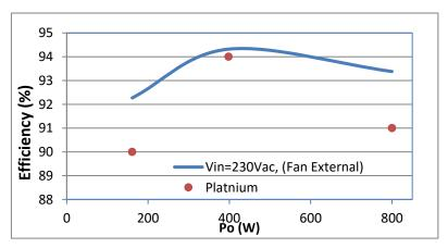
Figure 2. Efficiency vs. Load Current (Ratio Metric Loading)
