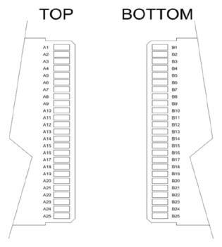
Figure 18. Pin Assignment of DC Connector
