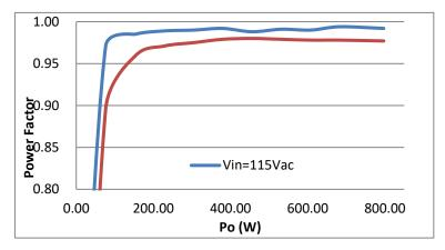
Figure 3. Power factor vs. Load current
