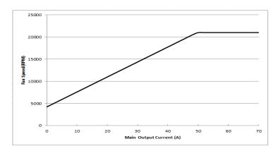
Figure 13. Fan speed vs. main output load
