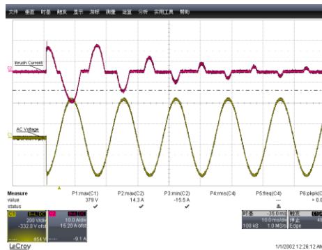
Figure 4. Inrush current, V_{in} = 264 \text{ VAC} , 90^\circ , CH1: V_{in} (200V/div), CH2: i_{in} (10A/div)
