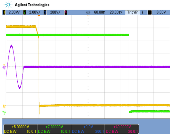
Figure 10. Turn-Off AC Line 230 VAC, full load (20 ms/div) CH1: V1 (2 V/div); CH2: VSB (2 V/div); CH3: Vin (200 V/div)
