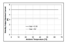
Figure 9. Current Limitation and Temperature Derating on 3.3 / 5 V<sub>SB</sub>
