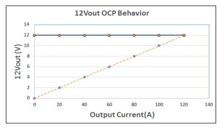
Figure 7. Current Limitation on V1
