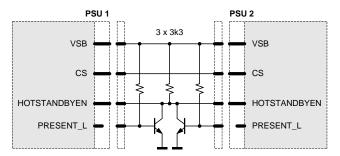
Figure 15. Recommended hot-standby configuration
