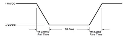
Figure 4. Minus 72 VDC Line Transient Test
