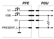
Figure 12. PRESENT\_L signal pin
