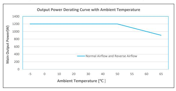
Figure 8. Derating Curve for ambient above 50°C
