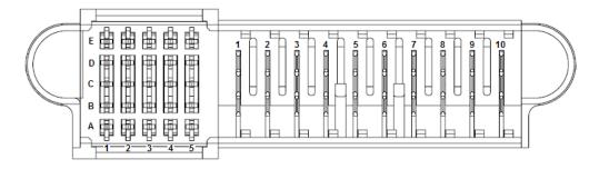
Power Supply Connector: Tyco Electronics P/N 2-1926736-3 **(NOTE: Column 5 is recessed (short pins))**Mating Connector: Tyco Electronics P/N 2-1926739-5 or FCI 10108888-R10253SLF
