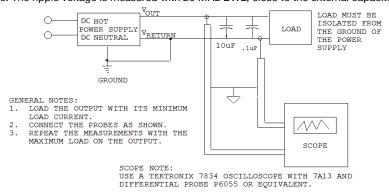
Figure 6. Output ripple test setup
