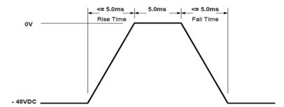
Figure 5. 0 V Line Transient Test
