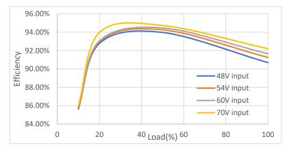
Figure 2. Efficiency Vs Load
