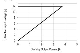
Figure 10. Current Limitation on 12 V<sub>SB</sub>
