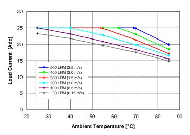
**Fig. 1:** Available load current vs. ambient air temperature and airflow rates for **QM48T25050** converter with B height pins mounted vertically with air flowing from pin 3 to pin 1, MOSFET temperature  $\leq$  120°C, Vin = 48 V.
