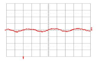
**Fig. 14:** Input reflected ripple current,  $i_s$  (10 mA/div), measured through 10  $\mu$ H at the source at full rated load current and Vin = 48 V. Refer to Fig. 13 for test setup. Time scale:  $1\mu$ s/div.
