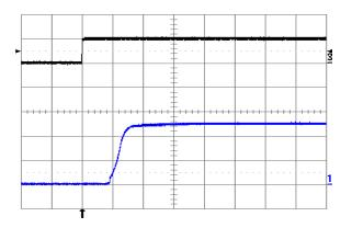
**Fig. 9:** Turn-on transient at full rated load current (resistive) with no output capacitor at Vin = 48 V, triggered via ON/OFF pin. Top trace: ON/OFF signal (5 V/div.). Bottom trace: output voltage (2 V/div.) Time scale: 2 ms/div.
