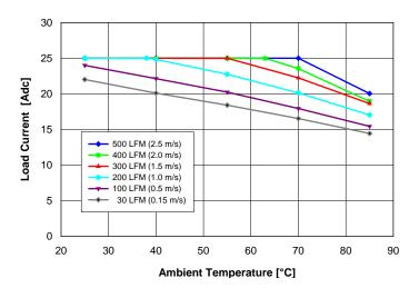
**Fig. 2:** Available load current vs. ambient air temperature and airflow rates for **QM48T25050** converter with B height pins mounted horizontally with air flowing from pin 3 to pin 1, MOSFET temperature  $\leq$  120°C, Vin = 48 V.
