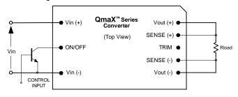
Fig. A: Circuit configuration for ON/OFF function.
