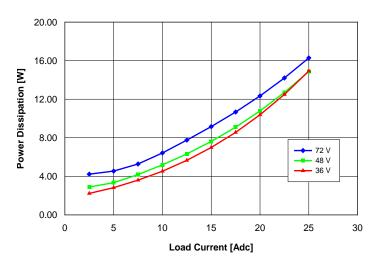
Fig. 7: Power dissipation vs. load current and input voltage for converter mounted vertically with air flowing from pin 3 to pin 1 at a rate of 300 LFM (1.5 m/s) and  $Ta = 25^{\circ}C$ .
