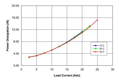
**Fig. 8:** Power dissipation vs. load current and ambient temperature for converter mounted vertically with Vin = 48 V and air flowing from pin 3 to pin 1 at a rate of 200 LFM (1.0 m/s).
