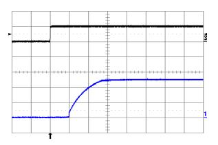
**Fig. 10:** Turn-on transient at full rated load current (resistive) plus 10,000  $\mu$ F at Vin = 48 V, triggered via ON/OFF pin. Top trace: ON/OFF signal (5 V/div.). Bottom trace: output voltage (2 V/div.). Time scale: 2 ms/div.
