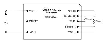
Fig. C: Configuration for increasing output voltage.
