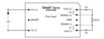
Fig. B: Remote sense circuit configuration.
