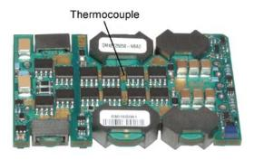
**Fig. H:** Location of the thermocouple for thermal testing.
