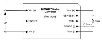
Fig. D: Configuration for decreasing output voltage.
