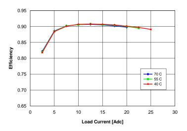
**Fig. 6:** Efficiency vs. load current and ambient temperature for converter mounted vertically with Vin = 48 V and air flowing from pin 3 to pin 1 at a rate of 200 LFM (1.0 m/s).
