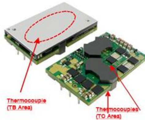
Figure 5. Location of the thermocouples for thermal testing
