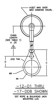
A NOTE THAT CHAIN LENGTH FOR SST ROPE WITH MOUNTING OPTION IS NOT MEASURED TO THE CENTER OF BULKHEAD MOUNTING LUG.
