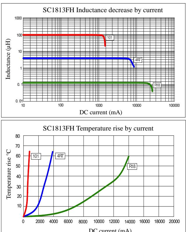
(1). Inductance tolerance for 0.18uH~1.6uH: ±30%, for 2.2uH~100uH: ±20%. Tested at 0.25V, 0ADC and 25°C.
