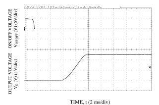
Figure 28. Start-up Using On/Off Voltage (lo = lo, max), Vo = 2.5 V
