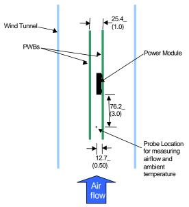
Figure 46. Thermal Test Setup
