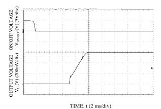
Figure 25. Start-up Using On/Off Voltage (lo = lo,max), Vo = 0.6 V
