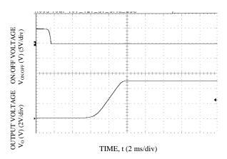
Figure 30. Start-up Using On/Off Voltage (lo = lo, max), Vo = 5.0 V
