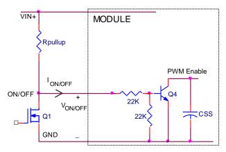
Figure 40. Circuit configuration for using negative On/Off logic
