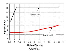
Output Voltage vs. Input Voltage Set Point Area plot showing limits where the output voltage can be set for different input voltages.
