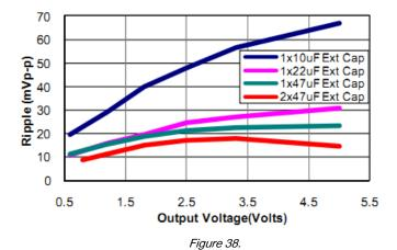
Note: Output ripple voltage for various output voltages with external 1x10  $\mu$ F, 1x22  $\mu$ F, 1x47  $\mu$ F and 2x47  $\mu$ F ceramic capacitors at the output (3 A load). Input voltage is 12 V.
