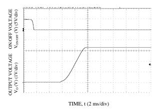
Figure 29. Start-up Using On/Off Voltage (lo = lo, max), Vo = 3.3 V
