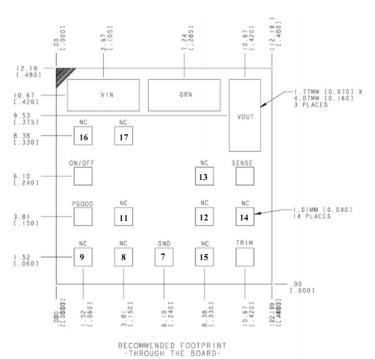
Figure 51. Recommended pad layout
