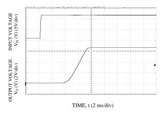
Figure 36. Start-up Using Input Voltage (VIN = 12 V, Io = Io,max), Vo = 5.0 V
