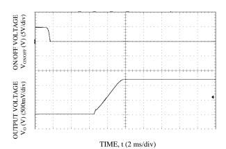
Figure 26. Start-up Using On/Off Voltage (lo = lo,max), Vo = 1.2 V
