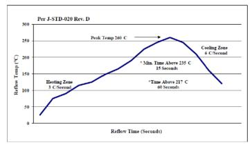
Figure 53. Recommended linear reflow profile using Sn/Ag/Cu solder
