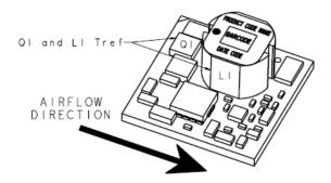
Figure 47. Preferred airflow direction and location of hot spot of the module (Tref)
