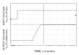
Figure 31. Start-up Using Input Voltage (VIN = 8 V, Io = Io,max ), Vo = 0.6 V
