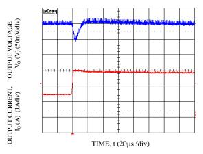
Figure 22. Transient Response to Dynamic Load Change from 50% to 100% at 12 Vin, Cout-2x47 μF, CTune-2700 pF & RTune-261 Ω. Vo = 2.5 V
