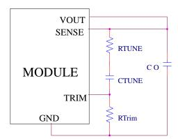
Figure 45. Circuit diagram showing connection of R<sub>TUNE</sub> and C<sub>TUNE</sub> to tune the control loop of the module
