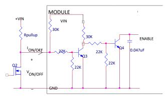
Figure 39. Circuit configuration for using positive On/Off logic
