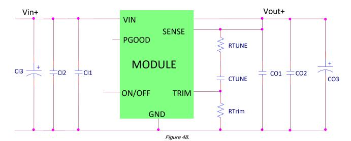
C11 Decoupling cap - 1x0.047 μF/16 V ceramic capacitor (e.g. Murata LLL185R71C473MA01)
