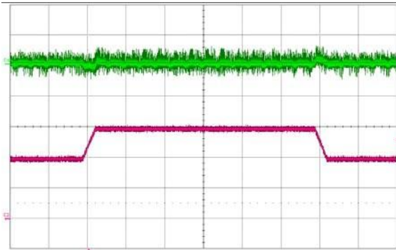
Figure 11. Output voltage response to load current step change (10 A – 15 A – 10 A) at V_{in} = 48 V. Top trace: output voltage (100 mV/div.) Bottom: load current (5 A/div.). Current slew rate: 0.1 A/μs. Time scale: 200 μs/div. C_o = 10 μF tantalum + 1 μF ceramic
