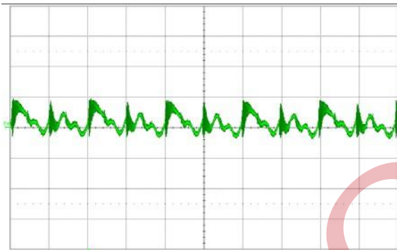
Figure 13. Output voltage ripple (20 mV/div.) at full rated load current into a resistive load with C_o = 10 μF tantalum + 1 μF ceramic and V_{in} = 48 V. Time scale: 2 μs/div.
