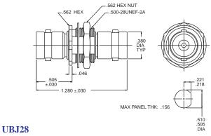
Bulkhead Jack Feed-Through, Insulated, 75 Ohm
