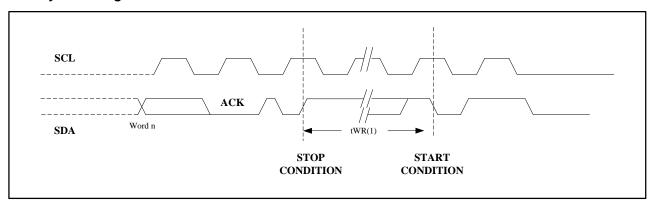
Figure 13. SCL: Serial Clock, SDA: Serial Data I/O
