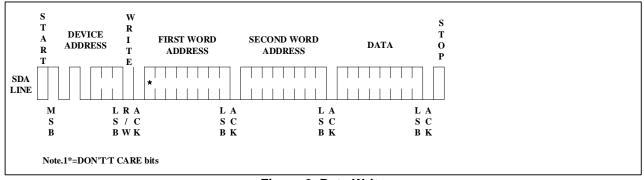
Figure 6. Byte Write
