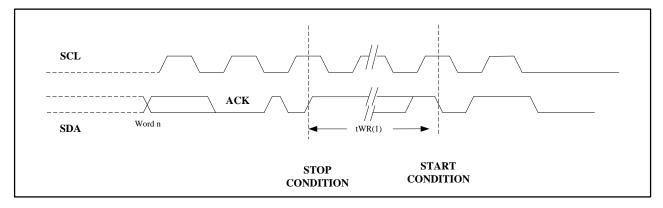
Figure 12. SCL: Serial Clock, SDA: Serial Data I/O
