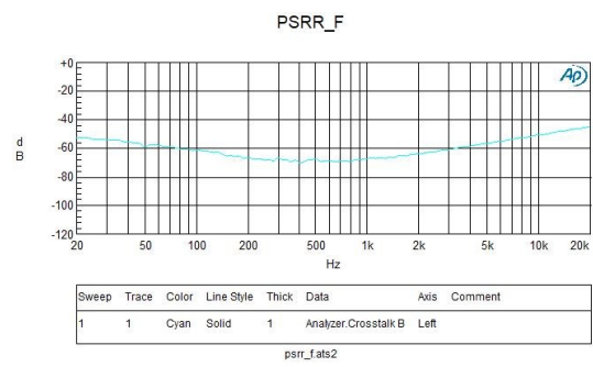
PSRR vs Frequency VDD=3V RL=8Ω
