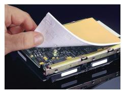
Gap Pad® VO is a cost-effective, thermally conductive interface material. The material is a filled, thermally conductive polymer supplied on a rubber-coated fiberglass carrier allowing for easy material handling. The conformable nature of Gap Pad® VO allows the pad to fill in air gaps between PC boards and heat sinks or a metal chassis.
