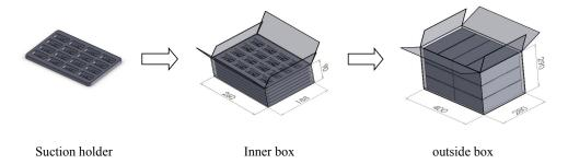
Packaging of Snap-in and Lead Types Supercapacitor:
