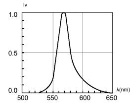
Fig. 1 Relative Luminous Intensity vs. Wavelength
