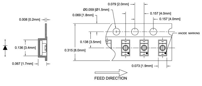
Outline Drawings Notes: 1. All dimensions are in inches [millimeters]. 2. Standard tolerance: ±0.010" unless otherwise noted.
