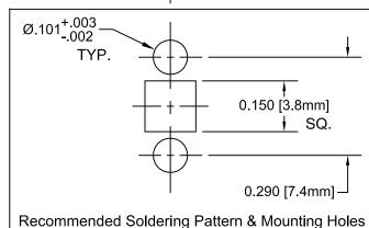
STANDARD TOLERANCE (UNLESS OTHERWISE SPECIFIED) **DECIMALS** ANGULAR ± .1  $X^{\circ}$  ± 1° TEL: (949) 951-8808 FAX: (949) 951-3974 .XX ± .02 TITLE: FLEXIBLE LIGHT-PIPE .XXX ± .010 SMD LED ADAPTER ASSY DESIGNED: PART NO: Brian Oliver 07/08/08 SMFLP5-X.X В CHECKED: CAGE CODE: 32559 | SHEET # 1 OF 1
