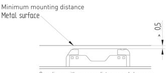
Compliance with creepage distances and clearances has to be ensured by the structural design of the luminaire.
