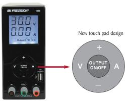
The model 1550 is a compact 108 watt power supply delivering  $1\text{-}36\ V$  and 0-3 A from its main isolated output. A unique feature of the 1550 supply is the USB charging port located on the front panel allowing the user to charge a cell phone or MP3 player. Clean power and quiet operation make this power supply ideal for any bench in laboratories, work shops and schools where bench space is limited.
