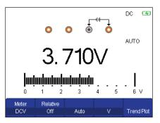
Speed up troubleshooting with the built-in 6000-count multimeter. Measurement functions include AC/DC voltage and current, resistance, capacitance, diode, and continuity test.
