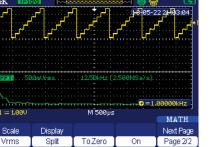
Display and measure the input signal's frequency spectrum. Select one of the 4 FFT windows: Rectangular, Hanning, Hamming, and Blackman. Use cursors to measure the spectral component's magnitude and frequency.
