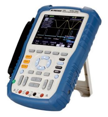
The 2510 Series handheld digital storage oscilloscopes provide floating measurement and recorder capabilities with a built-in digital multimeter (DMM), all in one portable and lightweight package. These versatile 60 MHz and 100 MHz bandwidth scopes offer 1 GSa/s sample rates, 2 Mpts waveform memory, 32 automatic measurements, and multiple recording functions to capture transient or long-term signal behavior.
