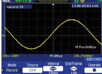
Monitor and analyze long-term signal behavior by recording data continuously over a period of time. These modes allow recorded data to be played back for post acquisition analysis.
