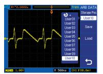
Store user arbitrary waveforms internally (up to 10 waveforms) or externally as an ARB or CSV file to a USB flash drive.
