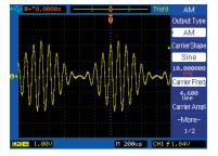
The built-in arbitrary waveform generator is capable of many different types of modulation for various applications. Modulate your waveforms with AM, FM, FSK, PSK, and PWM modulation schemes and use any of the 30 built-in waveforms as the modulating waveform.
